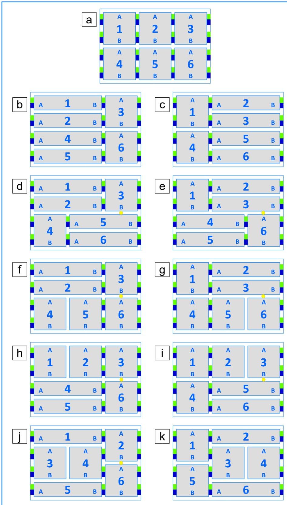
**Fig. 6 - Rocker combinations (EK-EH2-TP 6-function)**
